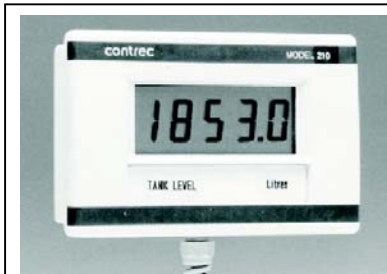
Fig 5. The Contrec 210 Loop powered indicator is IP67 for field or panel mounting. 24VDC Nominal Power is fed via 2 wires to the electronic level transmitter, which resolves the level in the tank as a 4-20mA signal in the loop. The 210 is installed in series into the 2-wire loop. It may be scaled 0-100% or In Engineering Units of contents if the vessel has a linear function.
