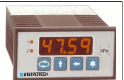
Fig 7. The Instrotech 4000 Series is a mains powered panel indicator, which provides the 24VDC supply to the level transmitter and provides the display functions as per the 210 in Fig 5. It is fitted with alarm/control contacts but if annunciation functions are required these are externally wired.
