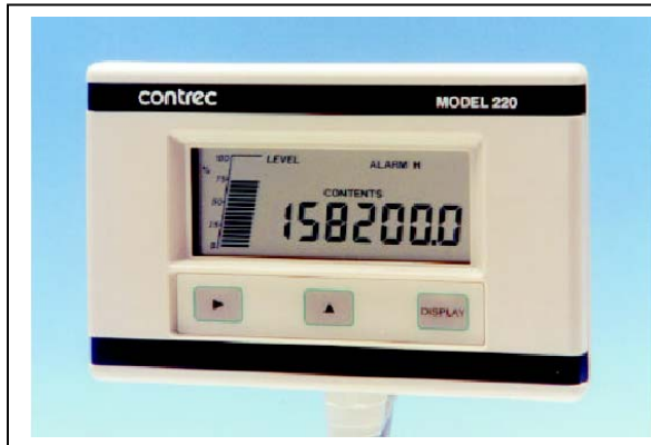
Fig 6. The Contrec 220 Level Monitor is also loop powered but can linearise the Tank Function, provide density correction, and has four switched outputs available for alarm and control functions. The alarm can be set to be acknowledged from a key on the fascia making this the ideal instrument for use at the fill point as required by AS1940.
